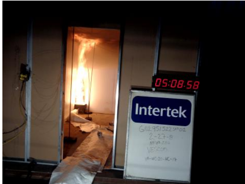
Photo No. 3 Increased Gas flow 160kW
