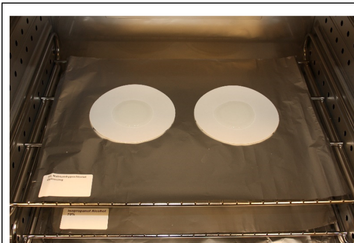
Specimen A: 3% Natrium hypochloriet solution – before the test.
