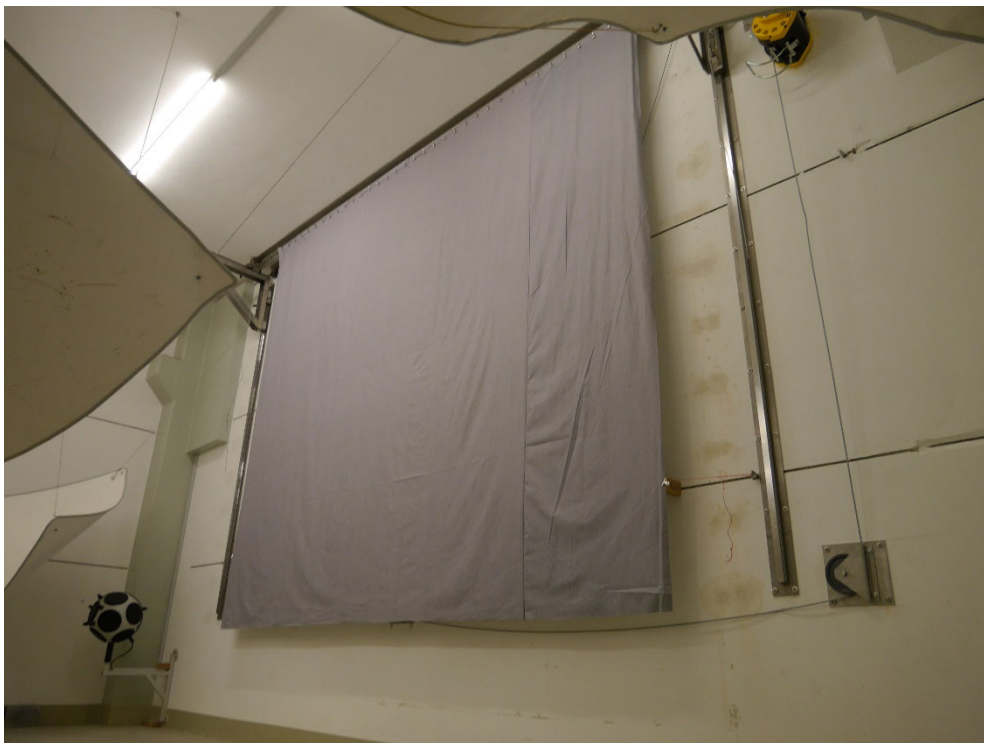
Figure B.2. Test object in the reverberation room: hanging flat, diagonal view.
