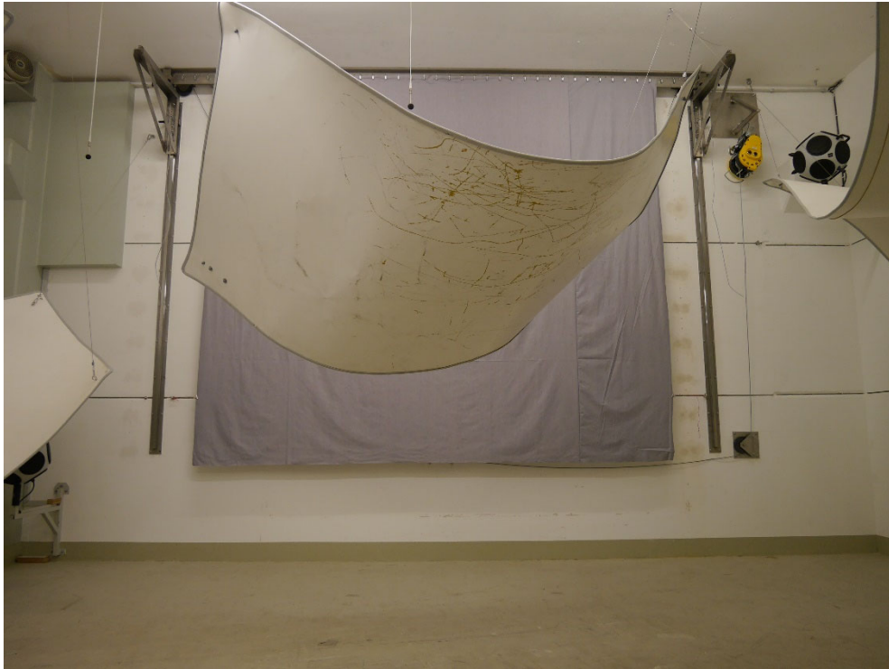
Figure B.1. Test object in the reverberation room: hanging flat, frontal view.
