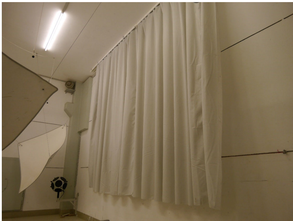
Figure B.4. Test object in the reverberation room: hanging rucked, diagonal view.
