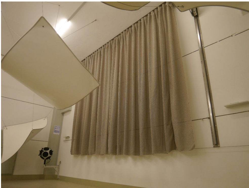
Figure B.4. Test object in the reverberation room: hanging pleated, diagonal view.
