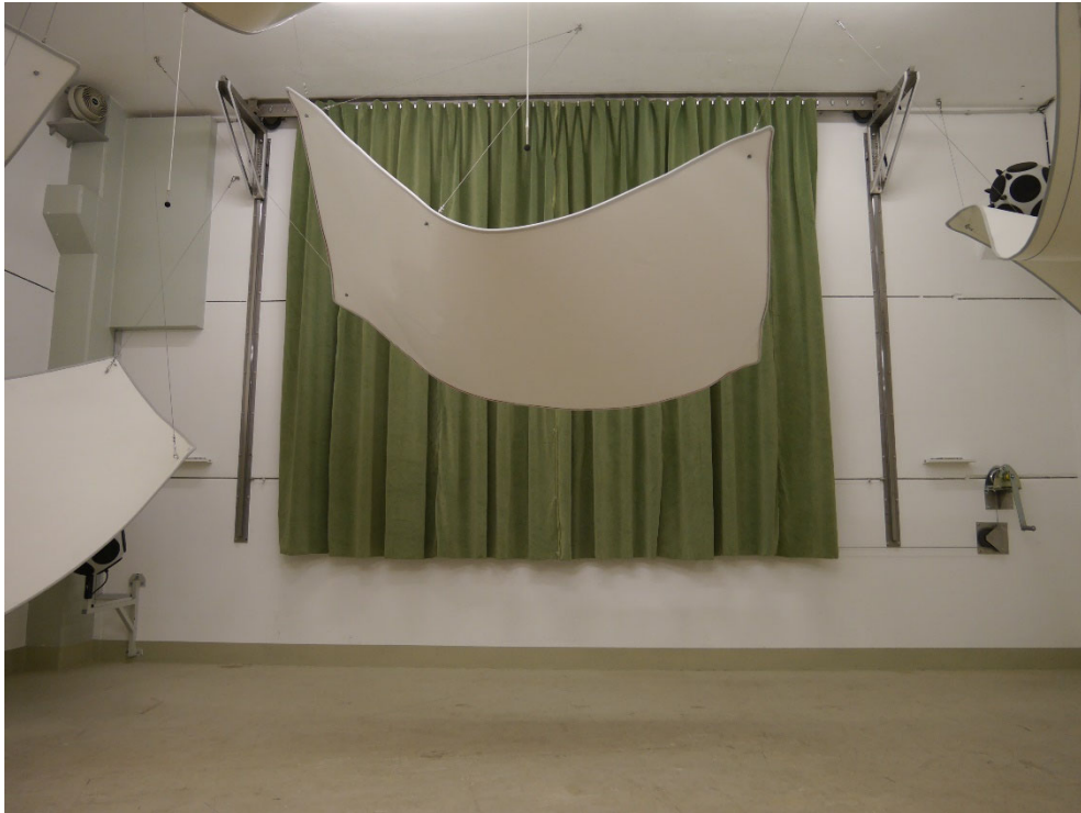
Figure B.3. Test object in the reverberation room: hanging pleated, frontal view.
