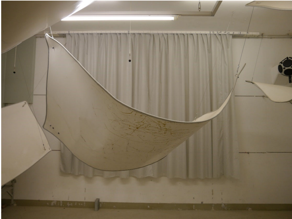
Figure B.3. Test object in the reverberation room: hanging rucked, frontal view.
