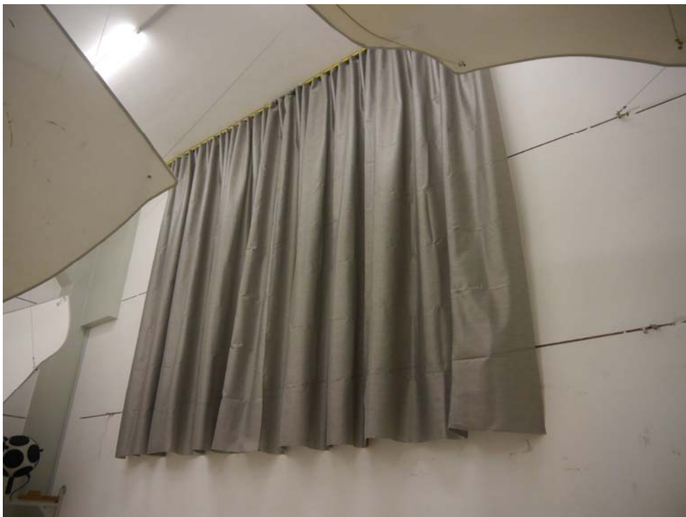
Figure B.4. Folded arrangement, test arrangement in the reverberation room: diagonal view.
