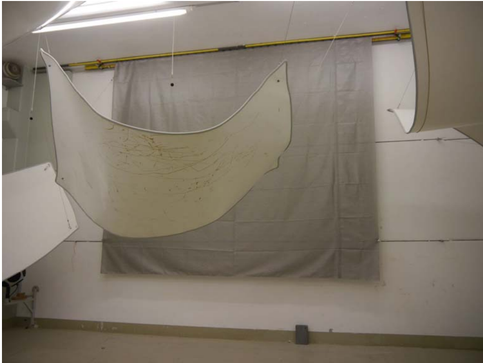
Figure B.1. Flat arrangement, test arrangement in the reverberation room: frontal view.
