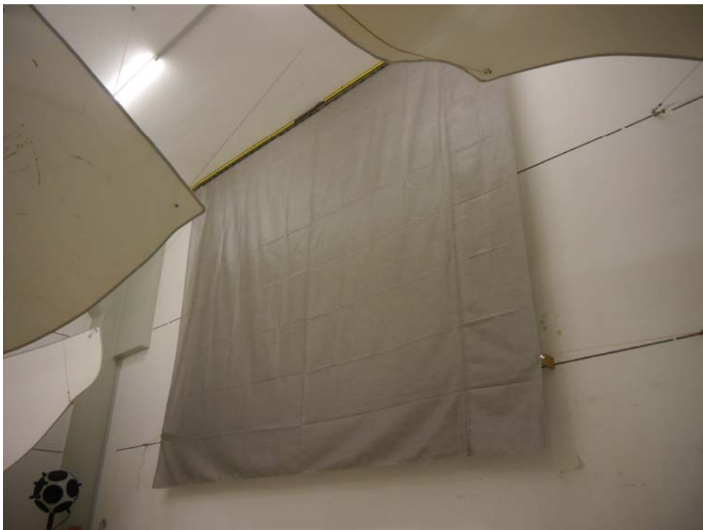
Figure B.2. Flat arrangement, test arrangement in the reverberation room: diagonal view.
