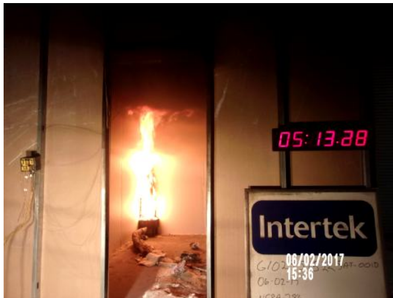
Photo No. 4 Gas flow 160kW
