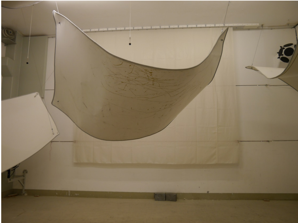
Figure B.1. Flat arrangement, test arrangement in the reverberation room.
