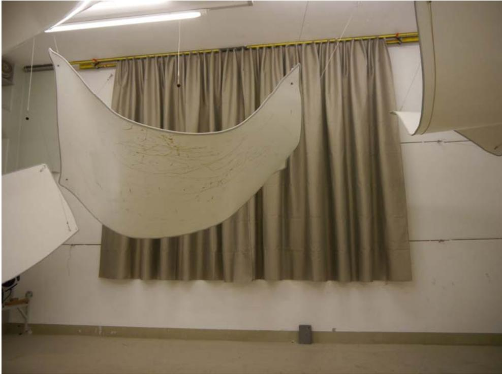
Figure B.3. Folded arrangement, test arrangement in the reverberation room: frontal view.
