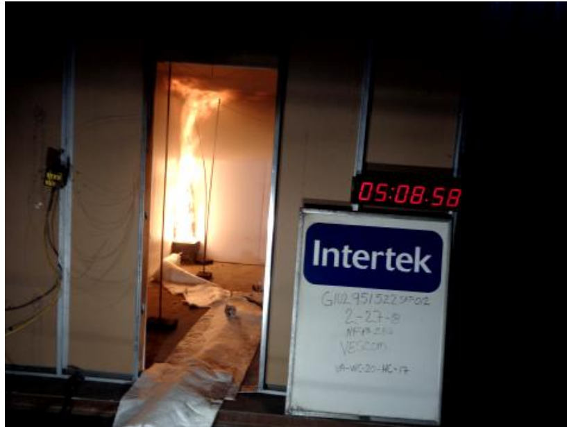
Photo No. 3 Increased Gas flow 160kW
