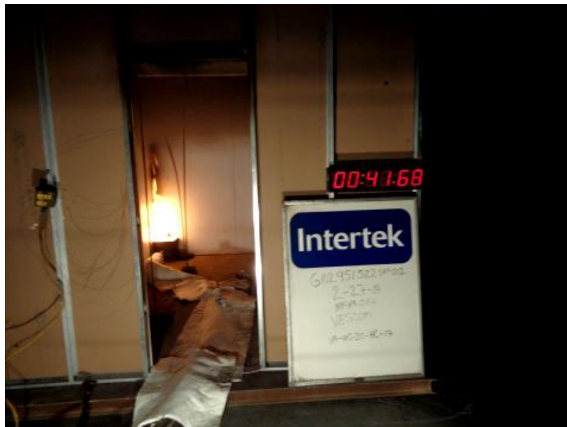
Photo No. 2 Start of test 40kW
