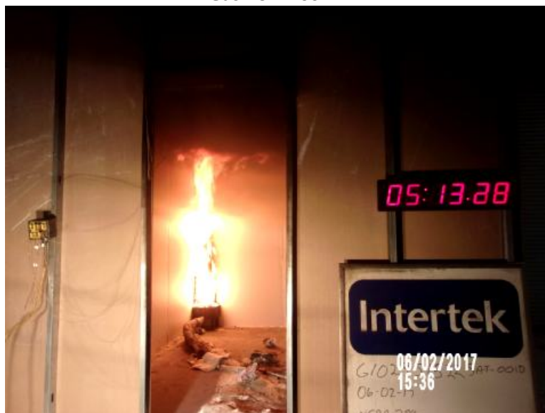
Photo No. 4 Gas flow 160kW
