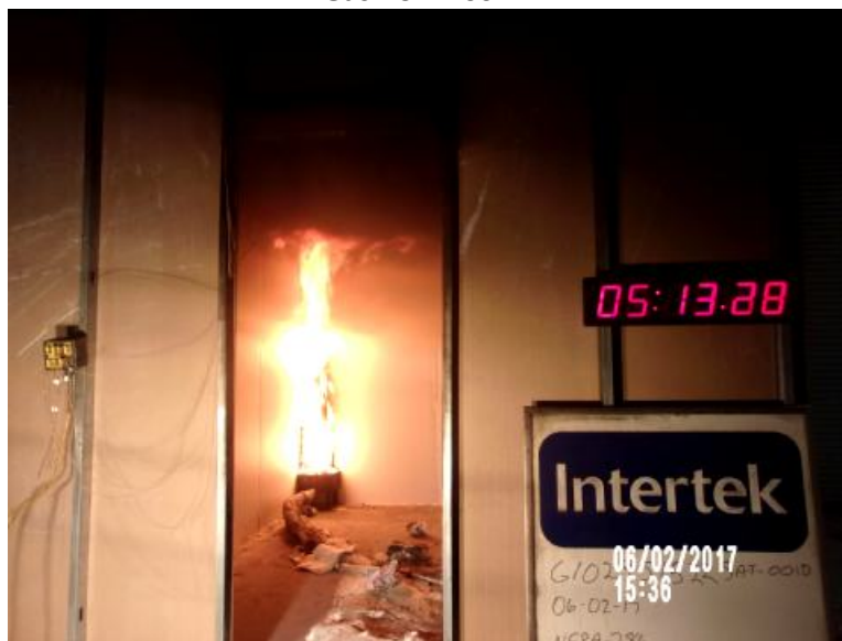
Photo No. 4 Gas flow 160kW
