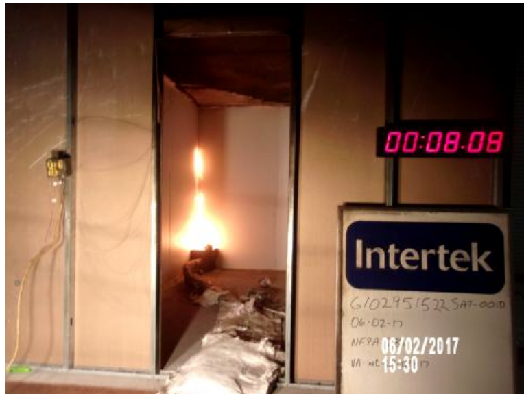
Photo No. 2 Start of test 40kW
