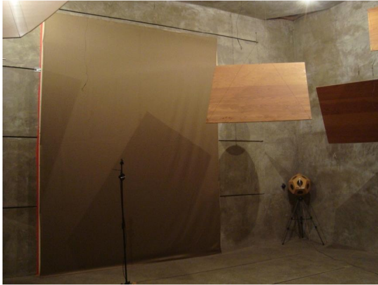
Figure 5.1: Measurement setup for determining the spectral sound absorption coefficient in the reverberation room at the specimen „Bedra“ suspended and plain
