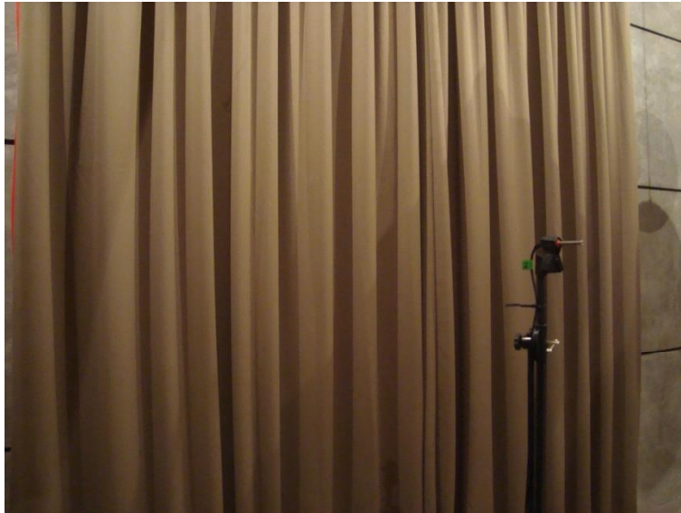
Figure 5.2: Measurement setup for determining the spectral sound absorption coefficient in the reverberation room at the specimen „Bedra“ suspended with tucks
