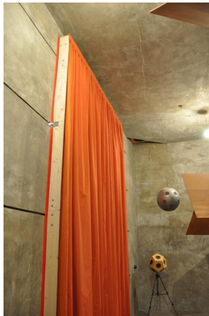
Figure 3.2: Measurement setup for determining the spectral sound absorption coefficient in the reverberation room; all-round frame with sealing tape
