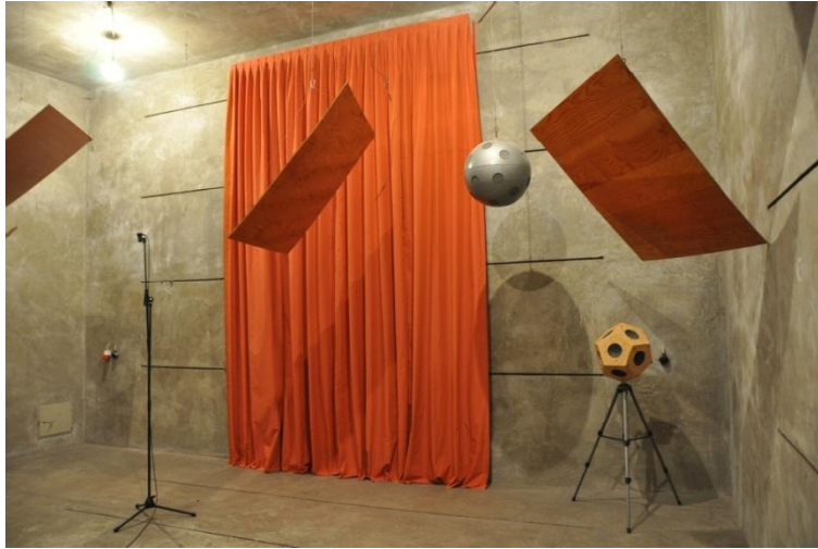
Figure 3.1: Measurement setup for determining the spectral sound absorption coefficient in the reverberation room
