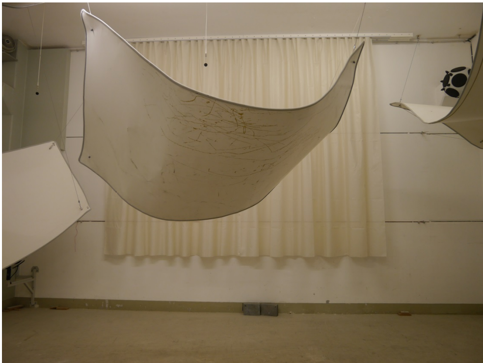
Figure B.2. Folded arrangement, test arrangement in the reverberation room.
